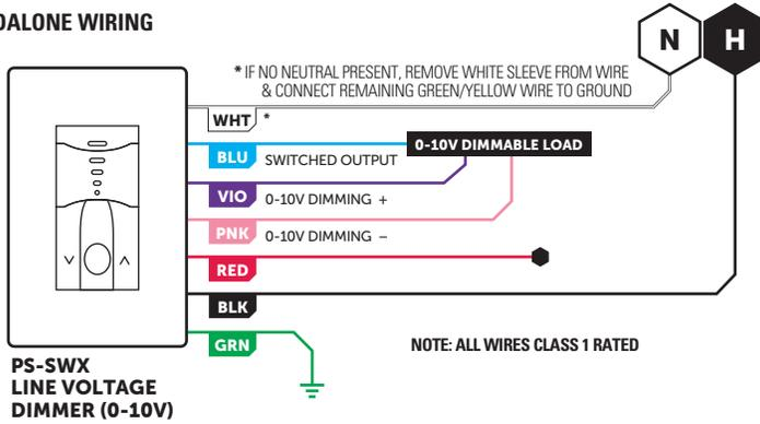
**NOTE: This product is UL listed and meets NEC 404.2(c) & 404.22 guidelines regarding powering over ground & current leakage. Powering over ground is permitted for replacement / retrofit only.**
